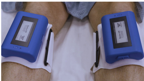
Fig. The RF Health MAC System (Recovery Force USA) is a lightweight (300-g) portable device. The dimensions of the device are 13.3 cm long, 8.9 cm wide, and 3.2 cm high. It is a wireless, portable, and wearable nonpneumatic device that allows for monitoring of the patient's movement, orientation, and activity. The device consists of a controller, which is mounted to the strap through a securement ring. A small DC (direct current) motor in the controller moves the securement ring in and out to contract and retract the strap.
